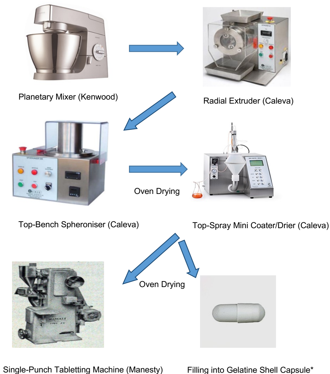
Figure 1.8: summarises the steps that conducted in this project for the overall process of making the coated pellets, where the pellets will be either filled into a capsule or compressed into a tablet. The shown images are similar to the equipment used in this project. *The scale-up of the capsule filling should consider the pellets feeder attached to the capsule filling machine. (Images were taken from the respective companies, except that the tableting machine image is taken from the gracesguide.co.uk , and the capsule image from www.naturalmedicines.co.uk ).
